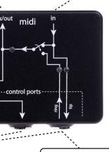
control port: This control port can also receive MIDI messages from an Empress pedal and send it to all the other outputs using a TRS cable. Be sure to set the internal dip switch on the midibox2 for this functionality.
