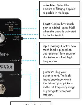
amp out: This buffered output can drive a long cable run without signal loss.
