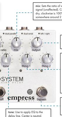
mix: Sets the ratio of wet signal (delay) to dry signal (unaffected). Counterclockwise is 100% dry, clockwise is 100% wet, with 50/50 being somewhere around 2 o'clock.
