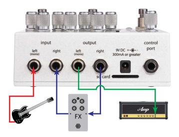
In this configuration the unit operates in mono. Left/right routing won't function as expected.
