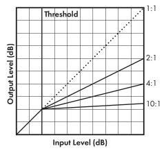
The **ratio** determines how much gain reduction will be applied to the signal once it crosses over the threshold. At a 4:1 ratio, for every 4dB of input signal above the threshold, there will be 1dB of output signal. A 10:1 ratio would output 1dB for every 10dB of input signal, etc.
